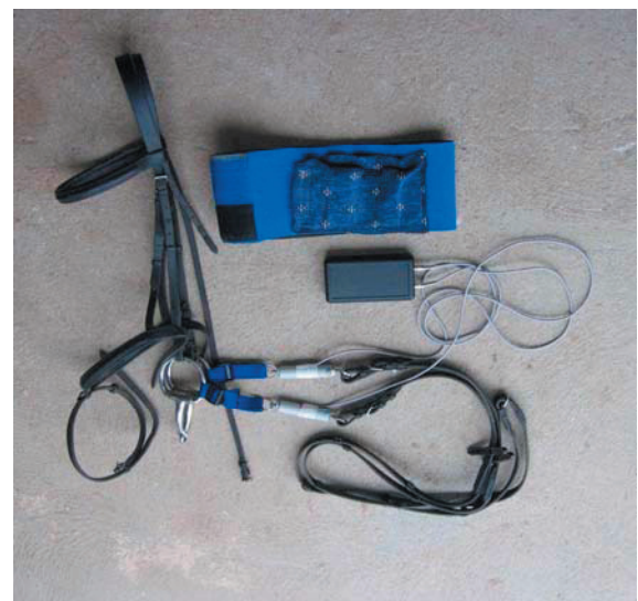
Figure 6. The Rein Gauge™ tensiometer currently being used in Australian studies. (Photograph with permission from Amanda Warren-Smith ).
